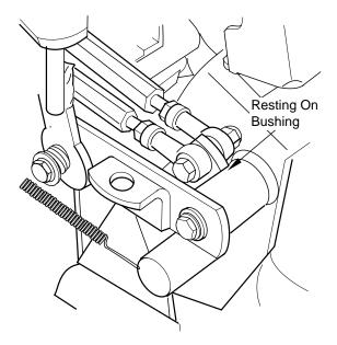
Figure 6-5 Bellcrank Touching Bushing
